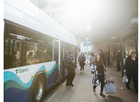
Entry and exit through multiple doors, level with the station platform
